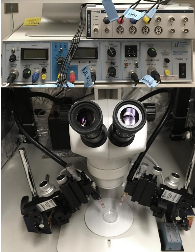
Figure 5. Apparatus for the measurement of the whole-cell currents of Xenopus oocytes using the two-electrode voltage clamp method. The voltage electrode and current electrode were placed on a micromanipulator and positioned over an oocyte, which was placed in a perfusion chamber. Both electrodes were connected to a feedback amplifier.
